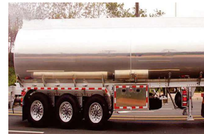
永强汽车制造有限公司——5083-H111、5454-H32铝合金板材 Oil tanker of YQ VEHICLES——5083-H111, 5454-H32 plate
